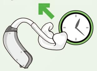
Wait until the earmold is completely dry before connecting it back together.
