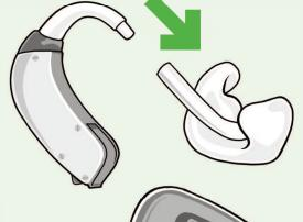
Disconnect the hearing aid by pulling it apart at the connection between the hook and tubing.
